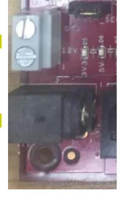
The S32R372141EVB supports two power options. You can generate 12V from a DC generator and connect that to P2; or you can plug in a 12V power supply through the barrel connector P1. NXP does not directly sell 12V power supplies. You can obtain a power supply through a third-party vendor.
