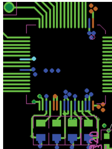
Figure 59. Top Layer Decoupling REFIN/REFOUT, REFCAPA, REFCAPB, and REGCAP Pins
