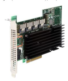
128 devices by leveraging SAS expander technology. Furthermore, the RS2WG160's SAS-2 architecture delivers data transfer rates of up to 6Gb/s per port, and brings new features and improved performance regardless of whether the storage solution utilizes 3Gb/s or 6Gb/s SAS or SATA drives.
