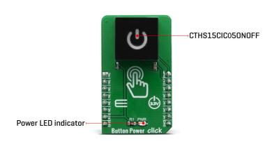
The power symbol icon on the top of the touch sensor is visible even when the backlight is off, thanks to the LEXAN™ polycarbonate film with an inverse print of the icon, placed on a top of the sensor. When the internal LEDs are turned ON, the light will pass through the translucent power symbol icon, resulting in a uniformly lit power symbol icon. An interesting lighting effect can be designed when touched, by applying a PWM signal to the IN pin.
