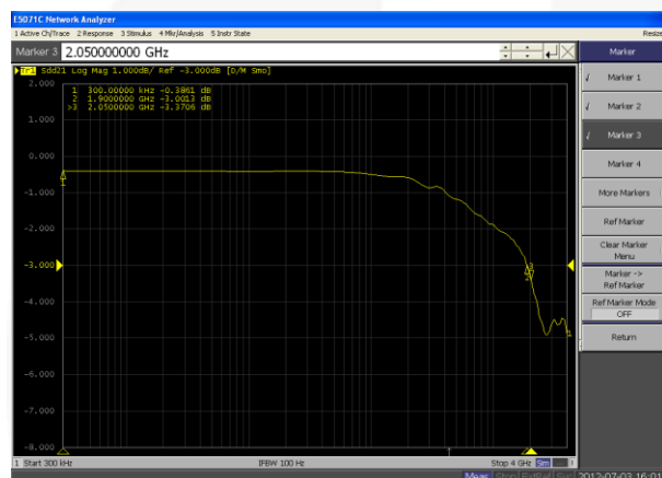
Figure 17. MHL Path SDD21 Insertion Loss Curve
