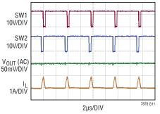
Pulse-Skipping Mode Waveforms with 100mA Load Buck Region (24V<sub>IN</sub>, 12V<sub>OUT</sub>)
