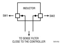
Figure 3. Sense Lines Placement with Inductor DCR
