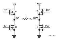
Figure 1. Simplified Diagram of the Output Switches
