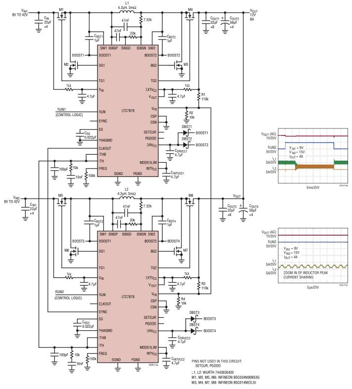
Figure 10. 12V<sub>OUT</sub>/8A Two-Phase Parallel Buck-Boost Converter with Different Inputs for Redundancy Design
