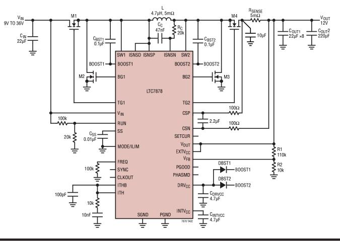
9V to 36V Input, 12V Output Buck-Boost Converter with 10A Output Current Limit
