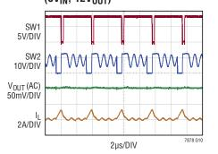
Pulse-Skipping Mode Waveforms with 100mA Load Buck-Boost Region (12V<sub>IN</sub>, 12V<sub>OUT</sub>)
