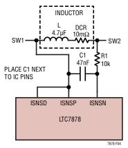
Figure 4. Inductor DCR Current Sensing
