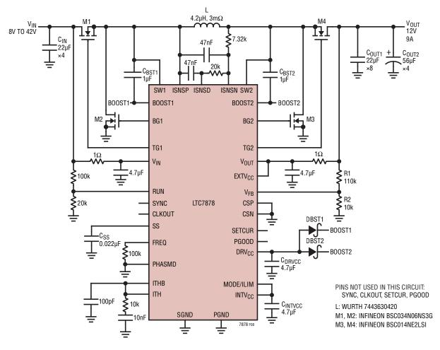
Figure 8. High Efficiency 8V to 42V Input, 12V<sub>OUT</sub>/9A Output Buck-Boost Converter
