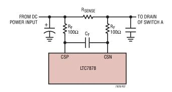
Figure 7. Programming Average Input Current Limit
