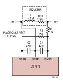
Figure 5. Small Inductor DCR Current Sensing
