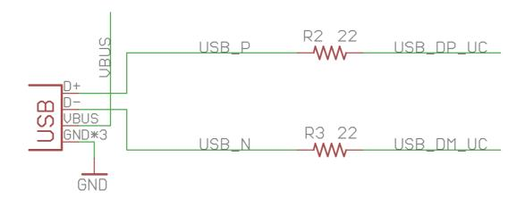
The USB data lines are terminated with 22 Ohm resistors. These data pins are also exposed via small through holes next to the USB connector and are labeled D+ and D-. The VBUS (+5VDC VCC of the USB port) is fed to the PMIC via a 3Amp Schottky diode (\$53P3). The VBUS pin is also available via the unpopulated header hole on the top-right side of the E series.
