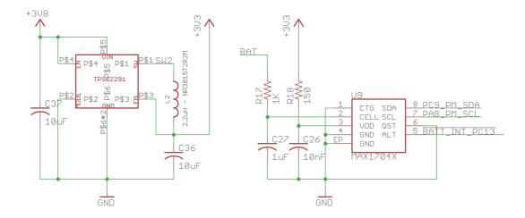
The output (3.8V net) of the PMIC is fed directly to the u-blox cellular module and a 3.3VDC high efficiency switching regulator (TPS62290). This 3.3VDC regulator helps power the microcontroller, fuel gauge and the buffers.
