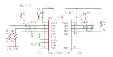
Since u-blox module's communication interface operates at 1.8VDC, while the STM32F205RGT6 microcontroller operates at 3.3VDC, we need voltage translators in-between them. This is achieved with two SN74AVC4T245 non-inverting buffers. The default state of the USART pins is set with the help of pull-up and pull-down resistors, and the unused input pins are tied to GND.
