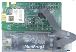
Fig 3: Programming/Debugging with MiniProg3
