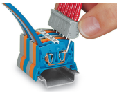
Testing by touch contact to the CAGE CLAMP® spring (limited to 0.5 A and 48 V test voltage) – test pins are not protected against accidental contact.
