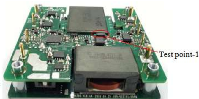
Figure 12 Temperature test points
