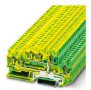
Protective conductor double-level terminal block, number of connections: 6, connection method: Spring-cage connection, 1st and 2nd level, Rated cross section:  $2.5~\text{mm}^2$ , cross section:  $0.08~\text{mm}^2$  -  $4~\text{mm}^2$ , mounting type: NS 35/7,5, NS 35/15, color: green-yellow
