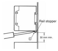
To remove the S82S from the DIN Rail, insert a screwdriver into section C and pull the S82S away from the Rail.
