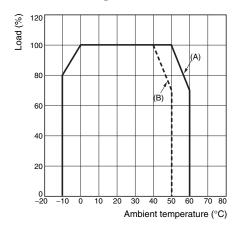
**Note:** The derating curve depends on the mounting direction of the Power Supply
