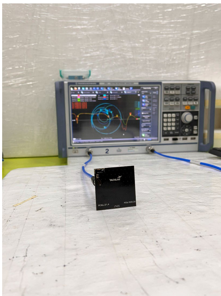
VNA Test Set-up on a 50x50mm Ground Plane
