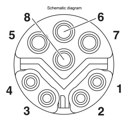
Pin assignment M12 socket, 8-pos.
