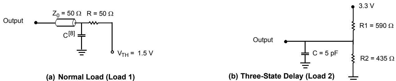
Figure 3. AC Test Load and Waveforms
