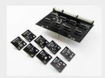
ROHM's sensor evaluation kit SensorShield-EVK-003 supports open platforms such as Arduino Uno, Lazurite, and mbed. Evaluation can be performed by combining 8 of ROHM's high-performance sensors.
