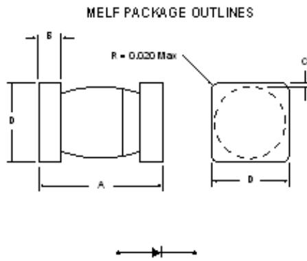
Note: Cathode side of device is indicated by a dark band marked on body.
