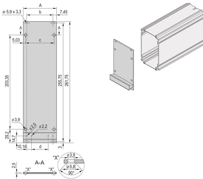
Front Panel for frame type plug-in unit, shieldable.
