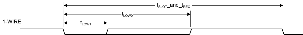
Figure 5-109. 1-Wire Write Bit Timing (Command/Address or Data)
