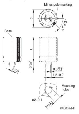
Snap-in terminals, length (6.3 ±1) mm. Also available in a shorter version with a length of (4.5 - 1) mm.
