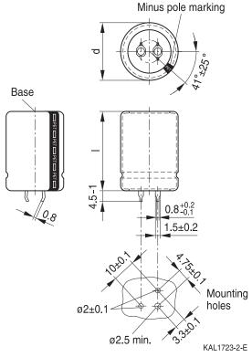
Snap-in capacitors are also available with 3 terminals (length (4.5 - 1) mm). Insulation is marked with "PET" on the sleeve. Safety vent on the base.
