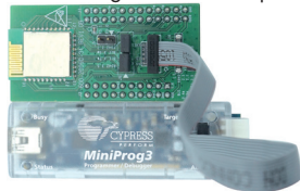
Fig 3: Programming/Debugging with MiniProg3
