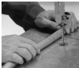
Position conduit at right-angle to band saw
