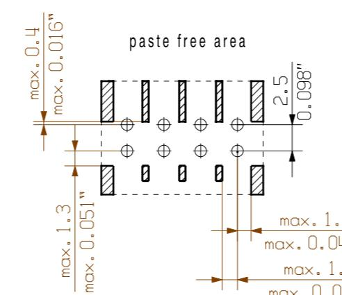
For the mounting of PCBs, it should be noted that the rated data given in the catalogue relates only to the connection elements. The necessary creepage and clearance paths must be observed in connection with the respective applicant in accordance to VDE 0110. The current-carrying capacity and pitch tolerance is to be determined according to DIN IEC 326 part 3 very fine.
