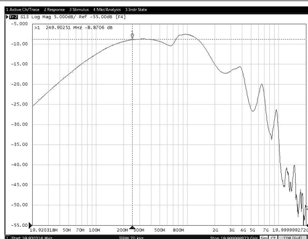
Figure 8-32. Off-State Data-Switch Isolation vs Frequency (TPS25830-Q1)
