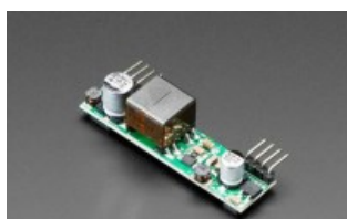
5V 1.8A Isolated Output PoE
