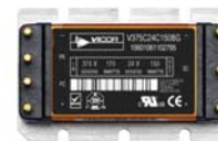
Micro converter example: V375C24C150BG 375 Vin, Micro, 24 Vout @ 150 W, long RoHS pins, slotted baseplate
