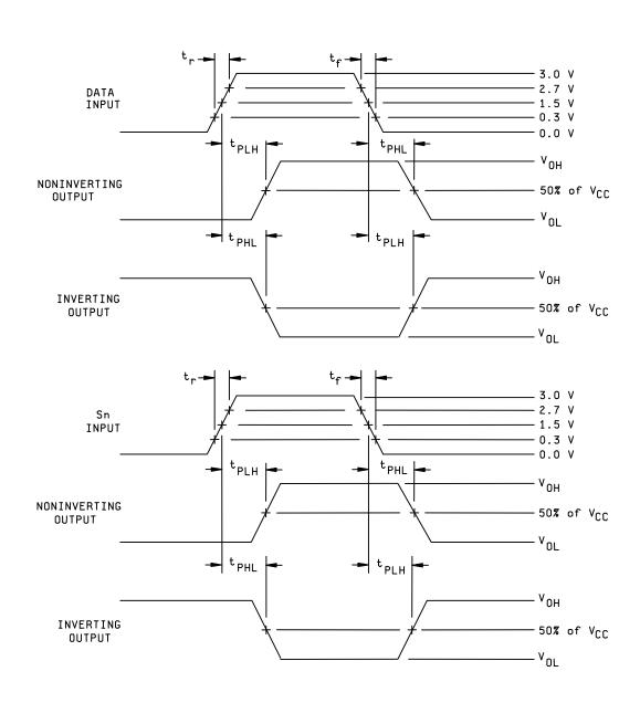
FIGURE 4. Switching waveforms and test circuit.
