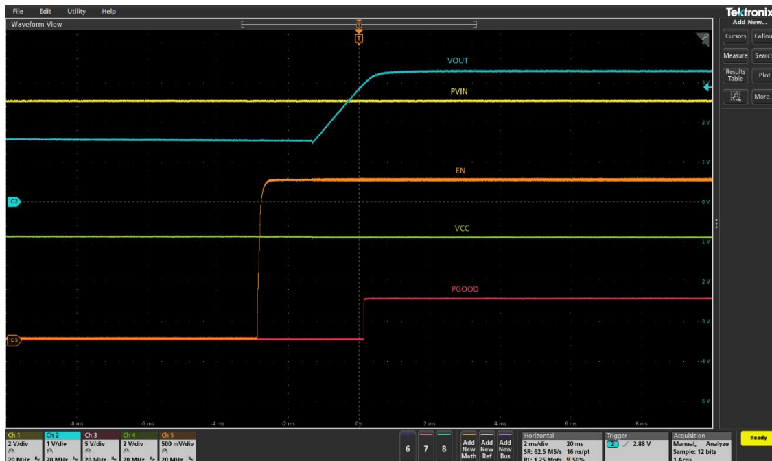
Figure 7 Startup into pre-bias (Ch1:PV IN , Ch2: V OUT , Ch3: PG, Ch4:V CC , Ch5: Enable)
