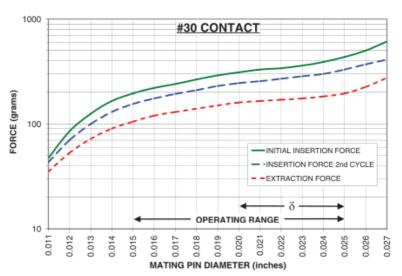
The insertion / extraction force characteristics above were derived using a 30 microinch gold-plated contact and polished steel gauge pins having a bullet-shaped tip.
