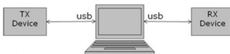
Figure 4. Connection setup 1: 1 PC with S2-LP-DK GUI
