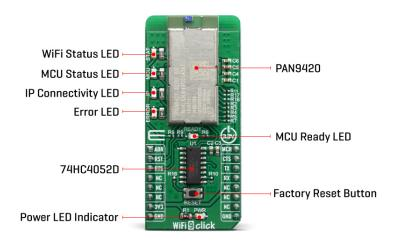
Parallel support of access point and infrastructure mode allows easy setup of simultaneous Wi-Fi connections from the module to smart devices and home network routers. The pre-programmed Wi-Fi SoC firmware enables client (STA), micro access point ( $\mu$ AP), and Ad-hoc mode (Wi-Fi Direct) applications. With the transparent mode, raw data can be sent from the UART to the air interface to smart devices, web servers, or PC applications.
