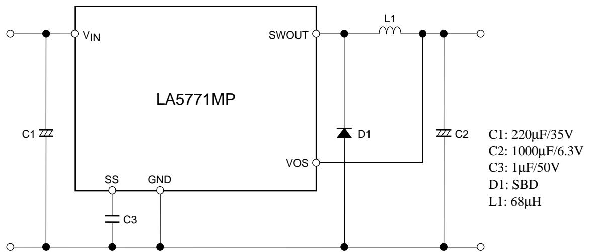
Notes: C3 is for the soft start function. Delete C3 and keep the SS pin open when the soft function is not necessary.
