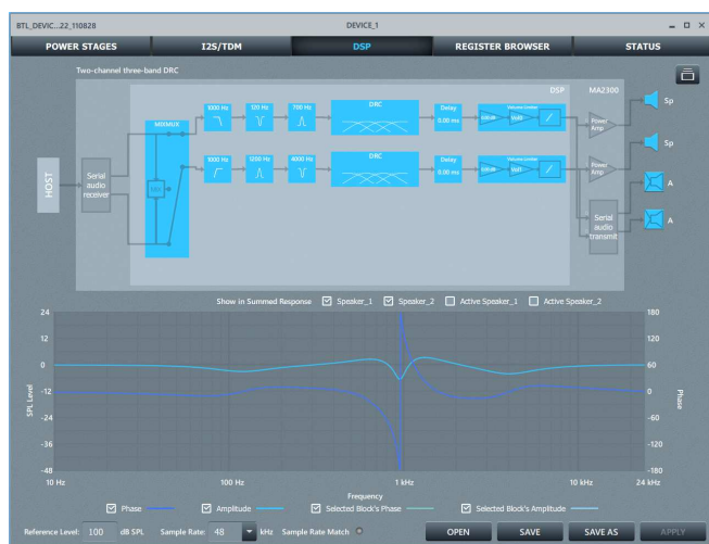
Figure 11.17: MA2304DNS GUI used for configuring the DSP
