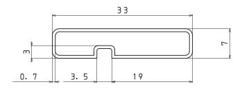
Tolerance=±0.3mm Thickness=0.7 $\pm$ 0.2mm Length =  $532.5 \pm 2$ mm Material = PVC (Antistatic treatment)
