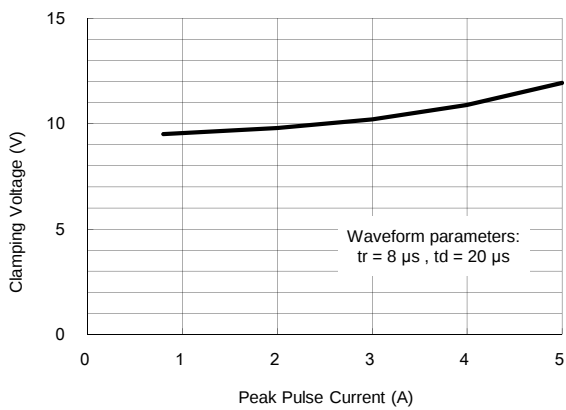
Fig. 3 Clamping Voltage VS. Peak Pulse Current
