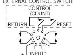
\* Note: Input polarity for DC operation. For most reliable operation on AC, connect high side to '+' and low side to '-'.
