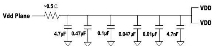
Figure 2. Recommended Power Supply Filtering
