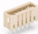
*Male header (for PCBs); Straight solder pin 1 x 1 mm; 2-pole; Pin spacing 3.5 mm / 0.138 in; 100% protected against mismating; with closed end; Vertical PCB mounting*
