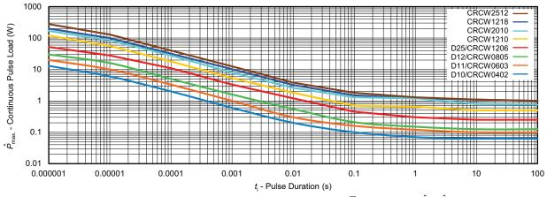
Maximum pulse load, continuous pulses; applicable if  $\overline{P} \le P(\mathcal{G}_{amb})$  and  $\hat{U} = \hat{U}_{max}$ ; for permissible resistance change equivalent to 8000 h operation
