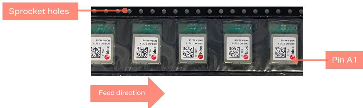
Figure 7: NORA-W306 module on tape orientation
