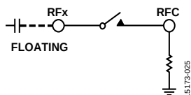
Figure 56. Series Capacitor Directly Connected to MEMS Switch
