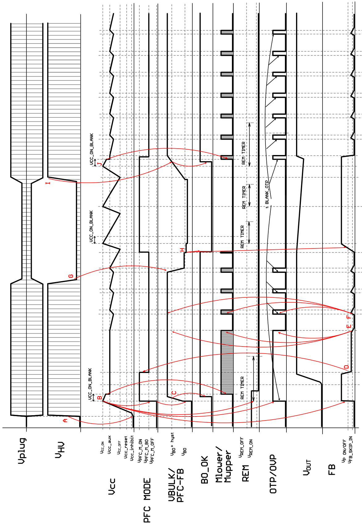
Figure 63. Startup, Skip-mode Operation, Low Lone Detection and Restart into Skip
