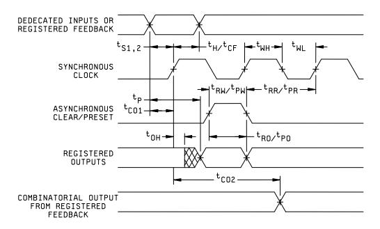
FIGURE 4. Switching waveforms.
