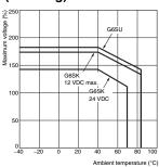
Note: "Maximum voltage" is the maximum voltage that can be applied to the Relay coil.
