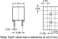
Note 1. Each value has a tolerance of ±0.3 mm. Note 2. The coplanarity of the terminals is 0.1 mm max.
