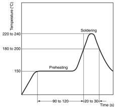
(The temperature profile indicates the temperature on the circuit board surface.)
