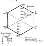
Conditions: Shock is applied in  $\pm X$ ,  $\pm Y$ , and ±Z directions three times each with and without energizing the Relays to check the number of contact malfunctions.
