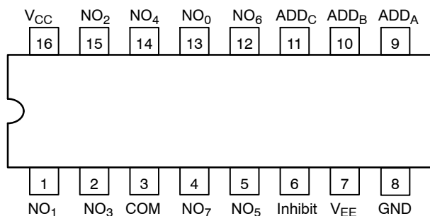
Figure 1. Pin Connection (Top View)
