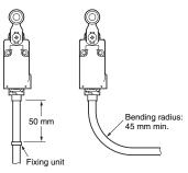
• When wiring, be sure to prevent penetration of a liquid such as water or oil through the cable end.
