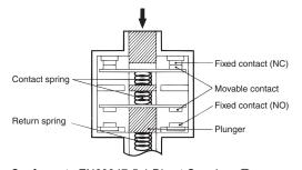
Conforms to EN60947-5-1 Direct Opening  $\bigcirc$ . (Only the NC contacts have a direct opening function.) When contact welding occurs, the NC contacts are separated from each other by pushing in the plunger.
