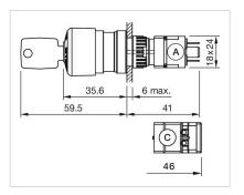
$\label{eq:Absolute} A = \text{Plug-in terminal } 2.8 \text{ mm x } 0.5 \text{ mm} \\ C = \text{Screw terminal}$
