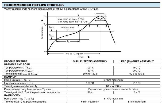
(1) For T27, lead (Pb)-free capacitors  $t_p = 30 \text{ s}$
