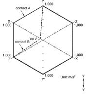
Sample: G6RN-1 24 VDC Number of Relays: 5 pcs Test conditions: The value at which malfunction occurred was measured after applying shock to the test piece 3 times each in 6 directions along 3 axes. Standard value: 100m/s² at contact A, 50m/s² at contact B
