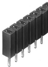
Female headers / BL 1 ... Stamped contact spring (fork contact), for □ 0.635 mm separable! any requested number...
