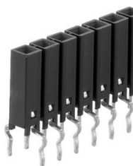
Female headers / BL 11 ... □ 0.635 mm, can be put through from above and below / 260 °C Reflow
